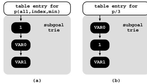
Fig. 7: Subgoal tries for  $p(X, I, Y)$  considering  $p/3$  declared (a) with and (b) without mode-directed tabling
