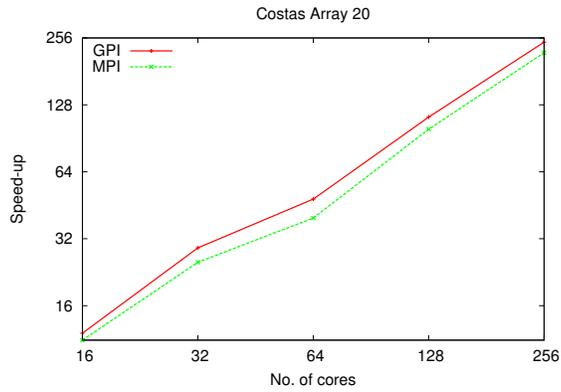
Fig. 2: Costas Array (n=20) on 256 cores (64 nodes)
